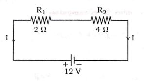
Calculate the equivalent resistance for the circuit which is connected to 12 V battery and also find the potential difference across 2  $\Omega$  and 4  $\Omega$  resistors in the circuit.
